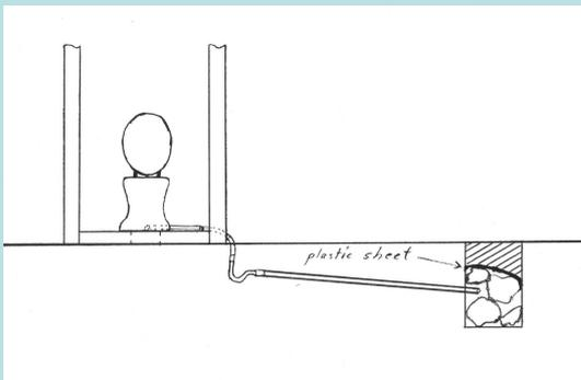
The connection of the „french-drain- set“ starts at the UDS-Bowl with the small L-BOW and the SHORT PIPE towards the side you want to have your french drain. The BIG L-BOW will go thru the hole in the toilet wall towards the P-TRAP which is outside and underground.
